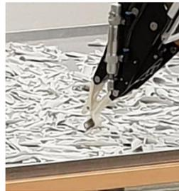
**Figure 2.2.** Grasping of the detected springs
